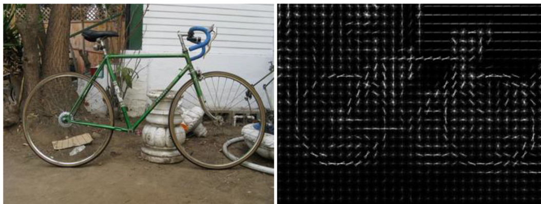
Fig. 1. Visualization of a Histogram of Gradients (HOG) object detector (right) for a given image (left). HOG captures the dominant gradients of the image (e.g. the bicycle) while ignoring near uniform areas (e.g. the area in the foreground).
